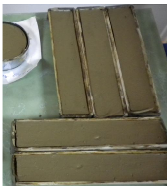
Fig. 2 – Samples during testing for the determination of linear shrinkage.
