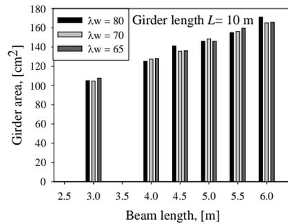
Fig. 6 – Design sensitivity of web slenderness,  $\lambda_w$ , with respect to the optimum area.
