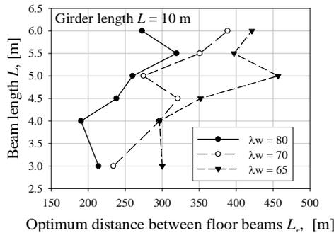
Fig. 5 – Design sensitivity of web slenderness,  $\lambda_w$ , with respect to the maximum distance between beam floors.
