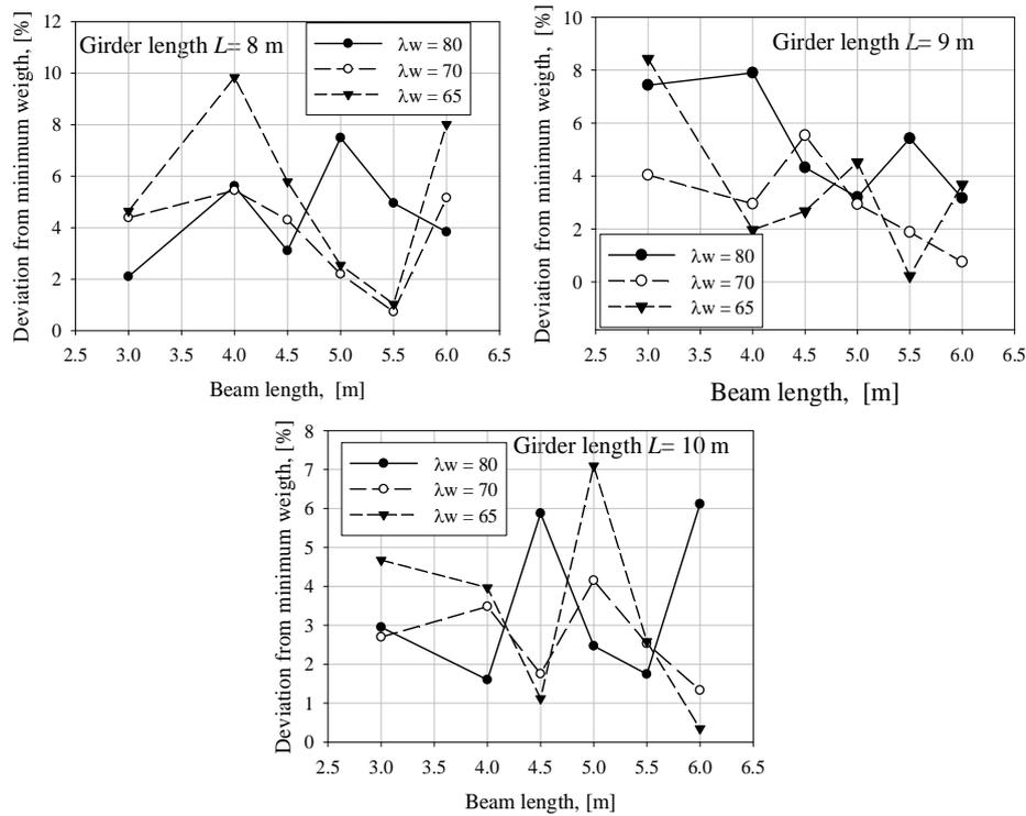
Fig. 4 – Design sensitivity of web slenderness,  $\lambda_w$ , with respect to the optimum girder weight.
