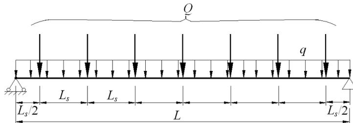
Fig. 3 – Imposed load and beam floor position on the girder.
