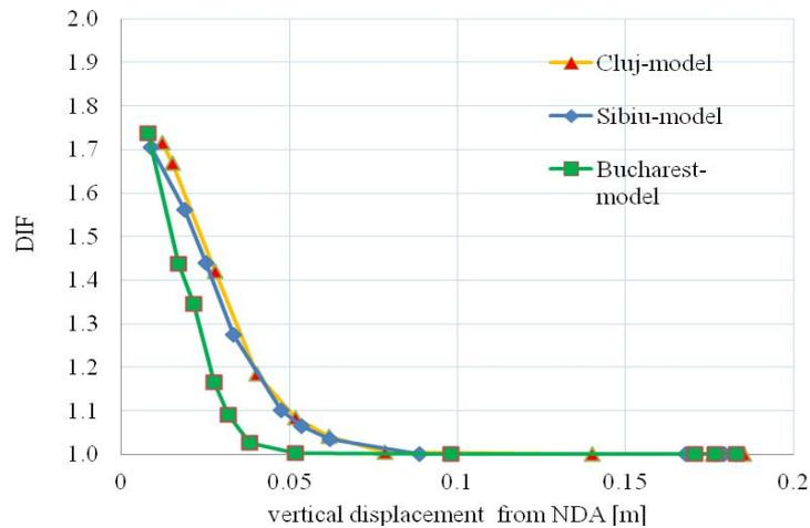
Fig. 6 – The estimated values of DIF based on the capacity curves of the models subjected to column-removal.
