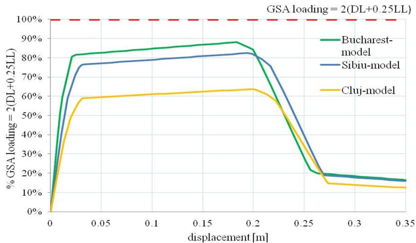
Fig. 3 – Load vs. displacement curves obtained from the nonlinear static analysis.
