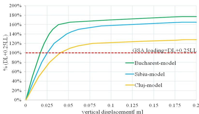
Fig. 7 – The influence of the seismic design on the ultimate load bearing capacity to progressive collapse of the six-storey RC framed structures.
