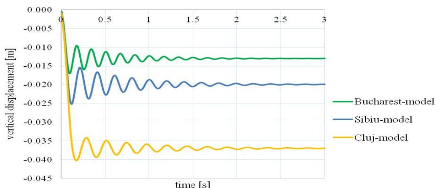
Fig. 4 – Time vs. displacement curves of the column-removed point obtained from the nonlinear dynamic analysis.
