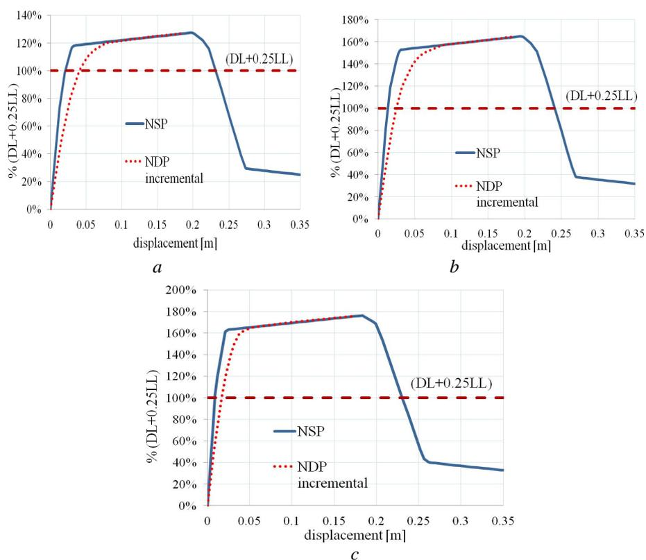
Fig. 5 – Load vs. displacement curves obtained with NS and ND incremental analyses: *a* – Cluj-model; *b* – Sibiu-model; *c* – Bucharest-model.
