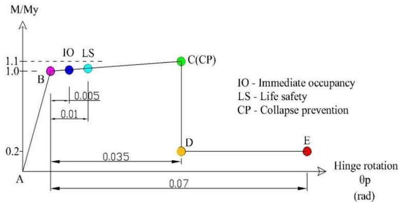
Fig. 2 – Plastic hinge model.
