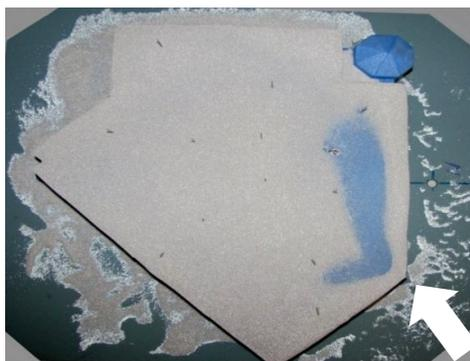
Fig. 5 – Snow drifted contours at the final experiment (wind direction is emphasized).
