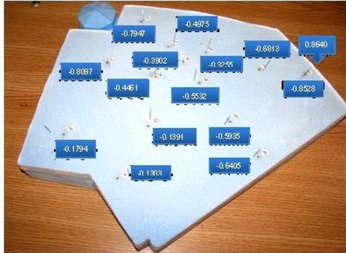
Fig. 1 – The model of the building and the positions of the pressure taps 1...15: top view with values of the local mean pressure coefficients.
