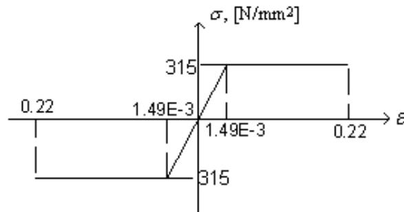
Fig. 2 – Strain–deformation relation.
