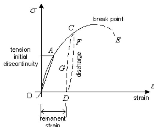
Fig. 3 – Typical “tension–deformation” curve for concrete.
