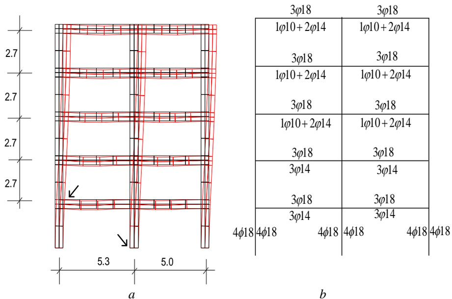
Fig. 1 – *a* – Digitization; *b* – the reinforcement of a reinforced concrete frame (5 levels).
