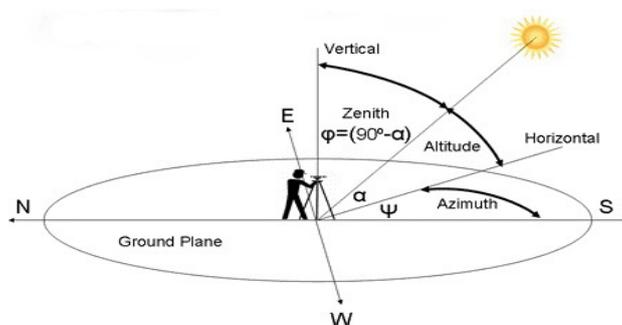
Fig. 2 – Azimuth and altitude for northern latitudes.
