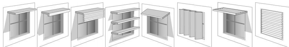
Fixed shading devices (Fig. 10), using correctly sized overhangs or porches, or design the building to be “self-shading” should be installed. Fixed
