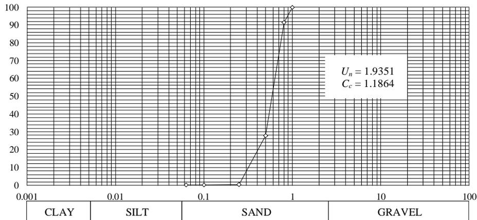
Fig. 4 – The grading curve of sand used for the laboratory tests.
