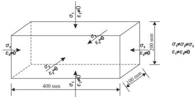
Fig. 3 – Sample sizes and stresses imposed in plane strain state (Cioară, 2012).
