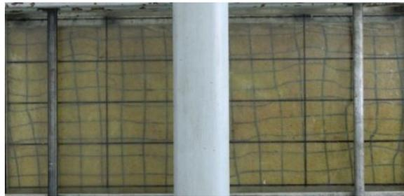
Fig. 9 – Failure of the second sample subjected to biaxial compression ( $\sigma_L = 80$  kPa).
