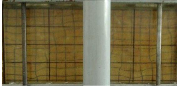
Fig. 8 – Failure of the first sample subjected to biaxial compression ( $\sigma_L = 50$  kPa).
