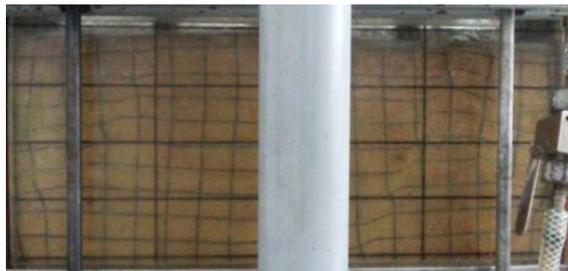
Fig. 10 – Failure of the third sample subjected to biaxial compression ( $\sigma_L = 110$  kPa).
