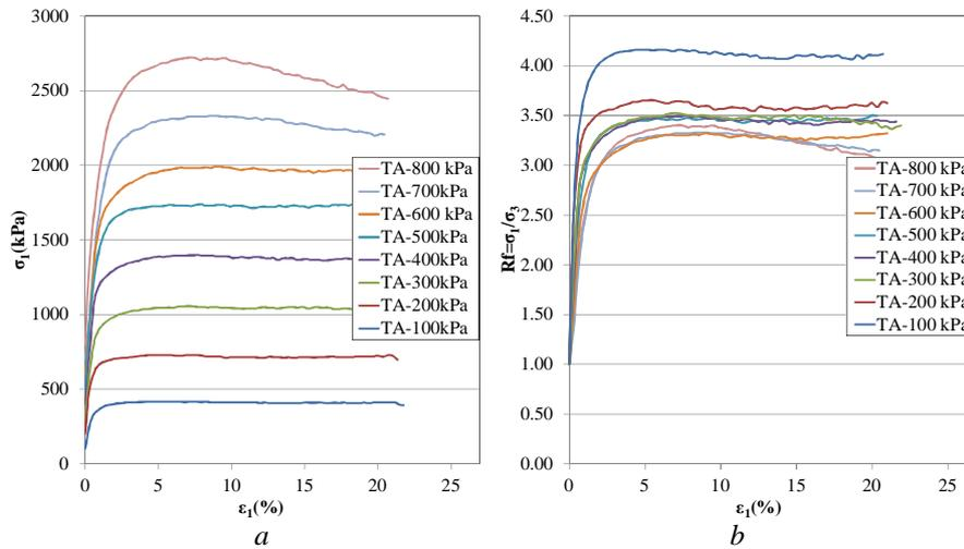
Fig. 6 – Stress–strain curves obtained from triaxial compression test: *a* – stress–strain curves; *b* – normalized stress–strain curves.
