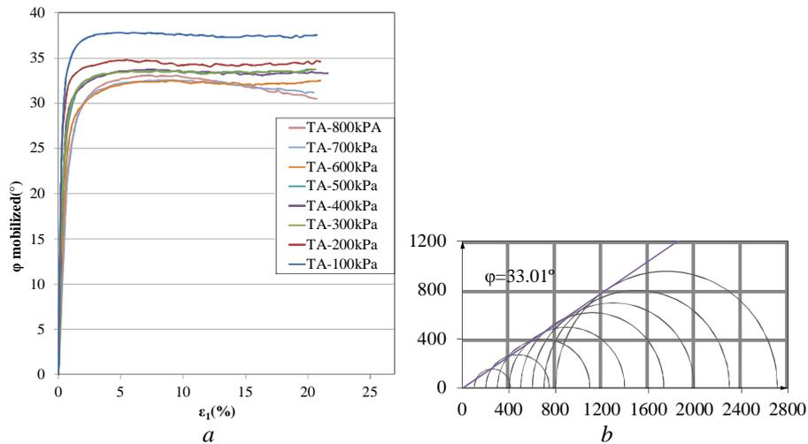
Fig. 7 – Value of the internal friction angle resulting from compression triaxial tests: *a* – curves of mobilization; *b* – limit circles and the intrinsic line.
