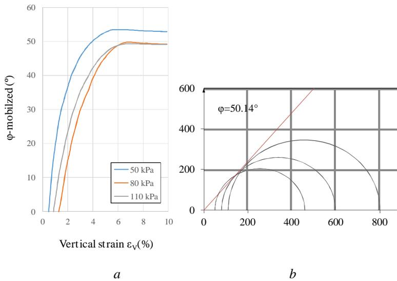
Fig. 12 – Internal friction angle values resulting from biaxial tests:
