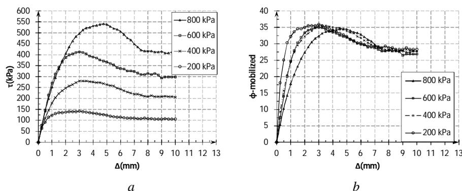
Fig. 5 – Relevant graphs obtained by direct shear testing: *a* – stress–displacement curves; *b* – internal friction angle mobilization curves.
