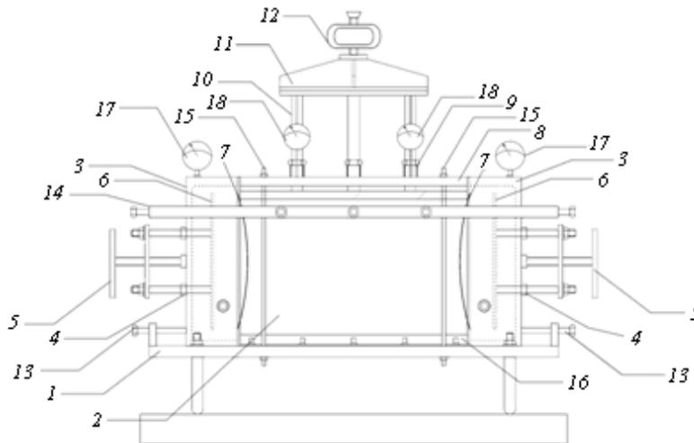
Fig. 2 – Original plane strain apparatus – biaxial cell details.
