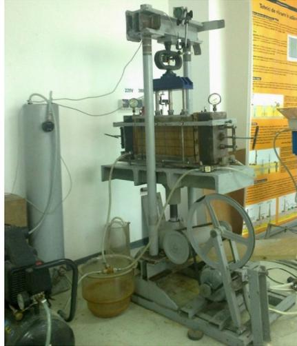
Fig.1 – Original plane strain apparatus (Stanciu, 1981).
