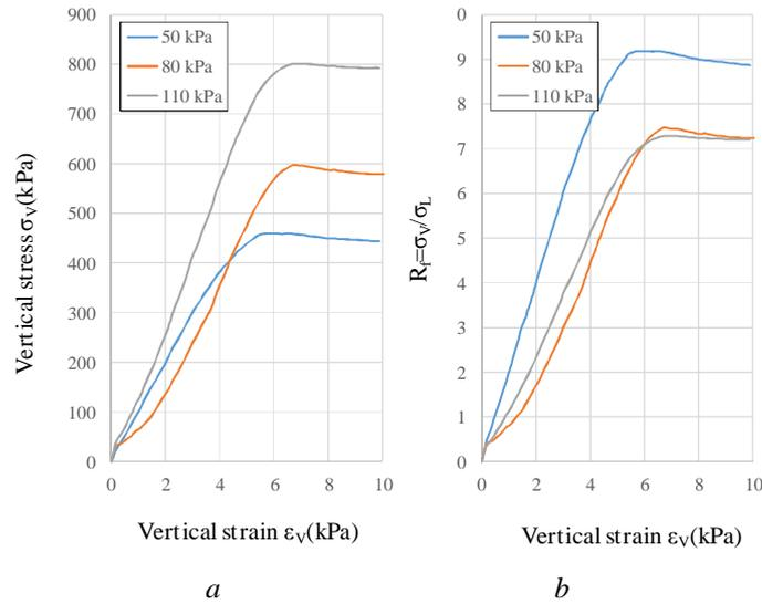
Fig. 11 – Stress–strain curves obtained from biaxial compression tests.
