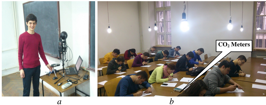
Fig. 1 – a – The equipments placed in the front part of the classroom (TESTO 480+SVANTEK 749); b – Photo during the tests.
