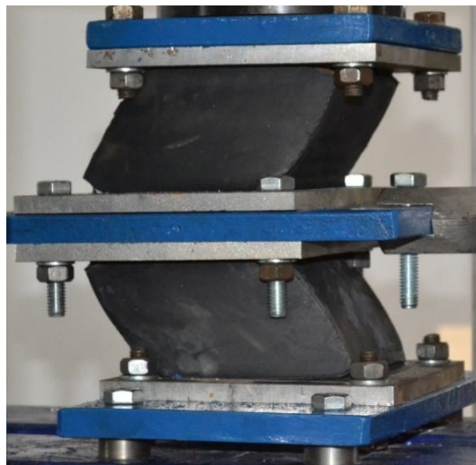
Fig. 8 – Elastomeric bearing degradation at 43 mm displacement.
