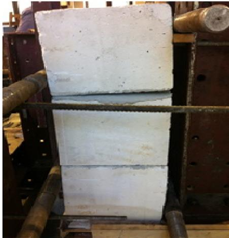
Fig.9 – Unreinforced masonry failure.
