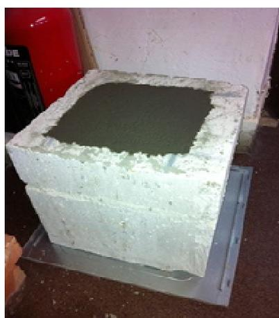
Fig. 2 – Sections made from confined disperse reinforced concrete BCA masonry.
