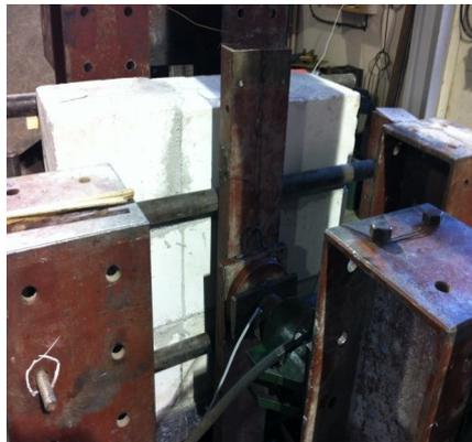
Fig. 7 – The bending strength of unreinforced masonry test.
