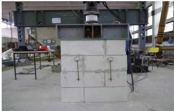
Fig. 12 – Compression tests on masonry sections.
