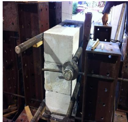
Fig. 8 – The bending strength of disperse reinforced confined masonry test.
