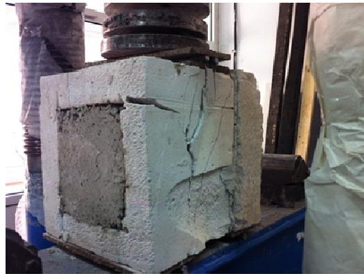
Fig. 4 – The failure of the metal fiber reinforced concrete masonry.
