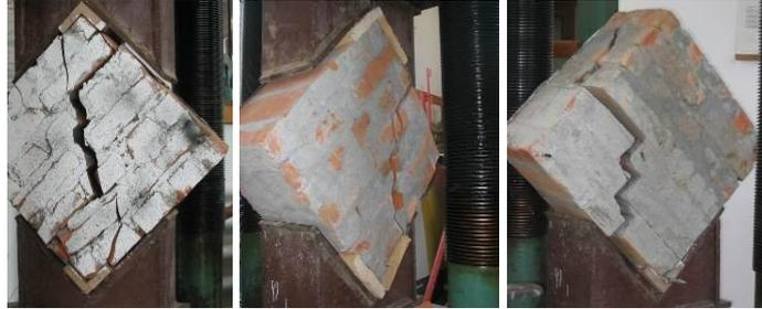
Fig. 9 – Damage pattern of one side retrofitted elements with SWM.
