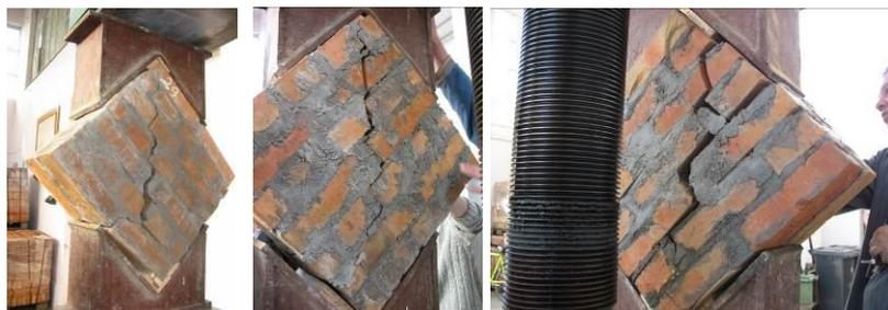
Fig. 8 – Damage pattern.
