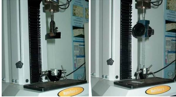
Fig. 5 – Tensile test on individual steel wire and steel meshes.
