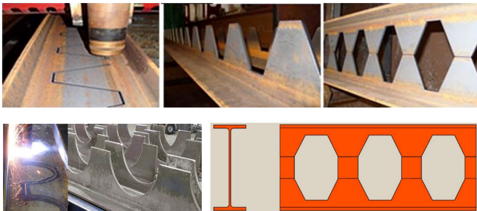
Fig. 2 – Cellular beams fabrication.
