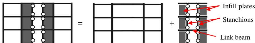
Fig. 1 – Dual SPSW with MRF, infill plates and stanchions.
