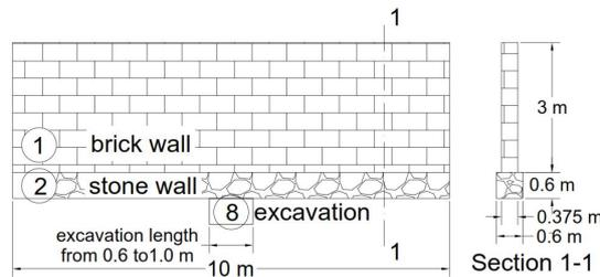
Fig. 2 – Detail of the excavation, with the wall and corresponding foundation.
