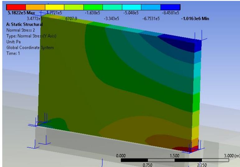
Fig. 5 – Typical in-plane stresses within the symmetrical model for the brick masonry wall – the excavation with 1 m length.
