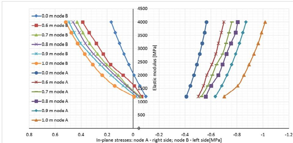
Fig. 6 – The evolution of the in-plane stresses correlated with the variation of the elastic modulus of the masonry wall for all the excavation lengths.
