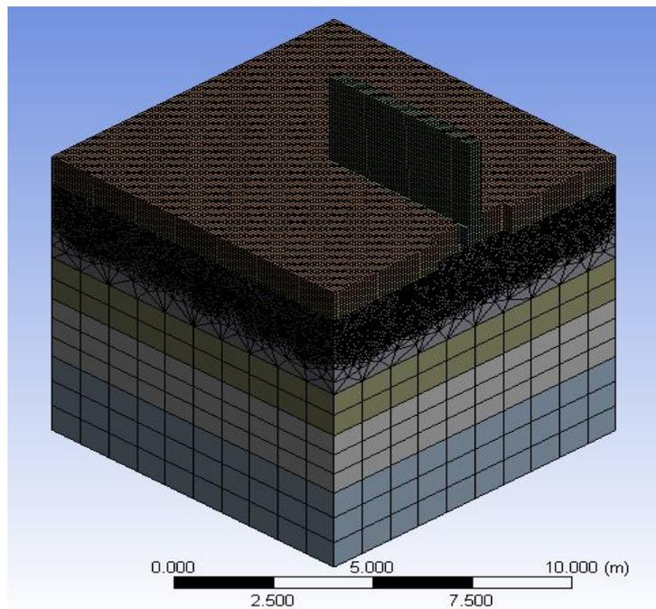
Fig. 4 – 3-D mesh pattern for the symmetrical geometry of the wall-foundation-soil system – the excavation with 1 m length.
