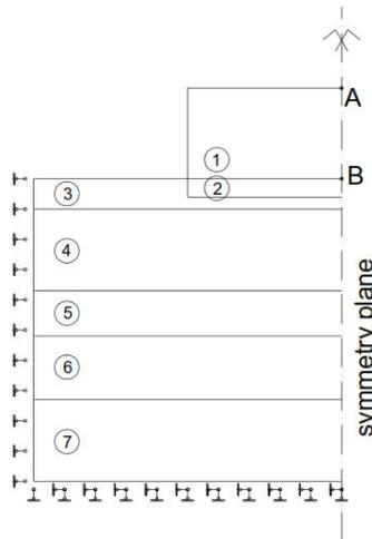
Fig. 3 – Applied symmetry on the wall – foundation system with restrains against displacements.
