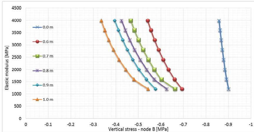
Fig. 7 – The evolution of the vertical stresses correlated with the variation of the elastic modulus of the masonry wall for all the excavation lengths.
