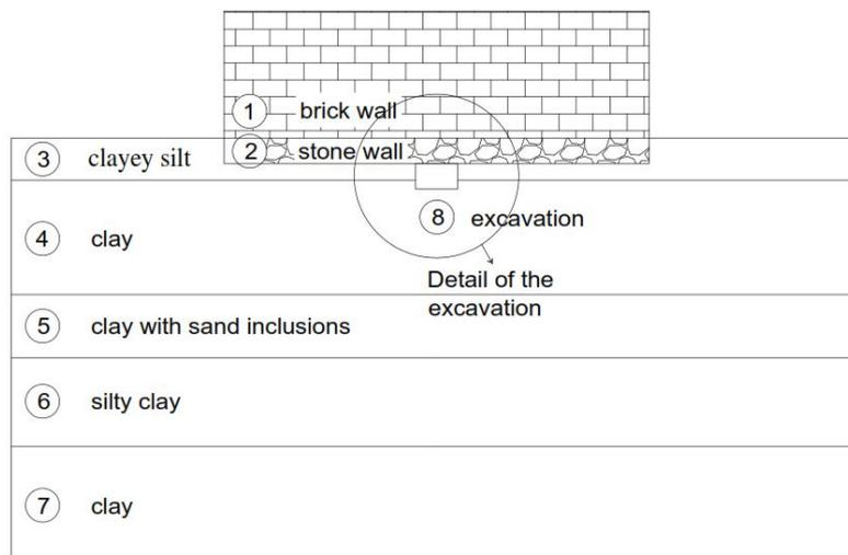
Fig. 1 – The model geometry – lateral view.
