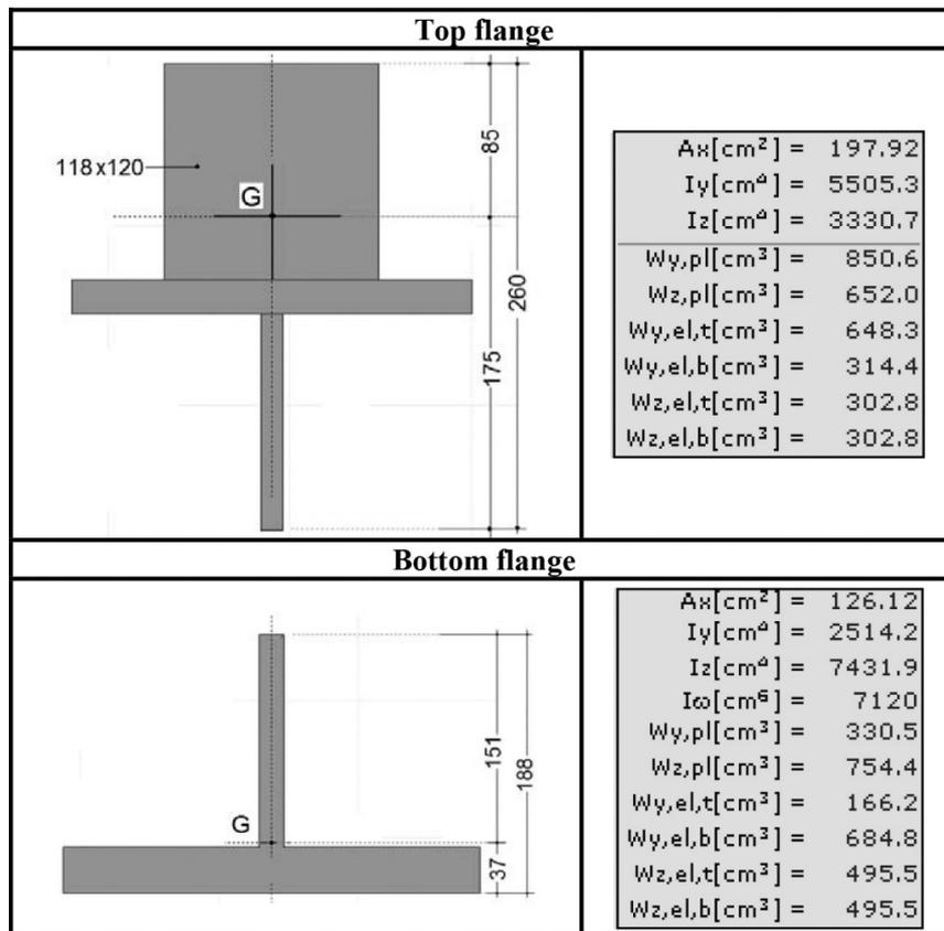
Fig. 7 – Flanges characteristics of the composite girder.
