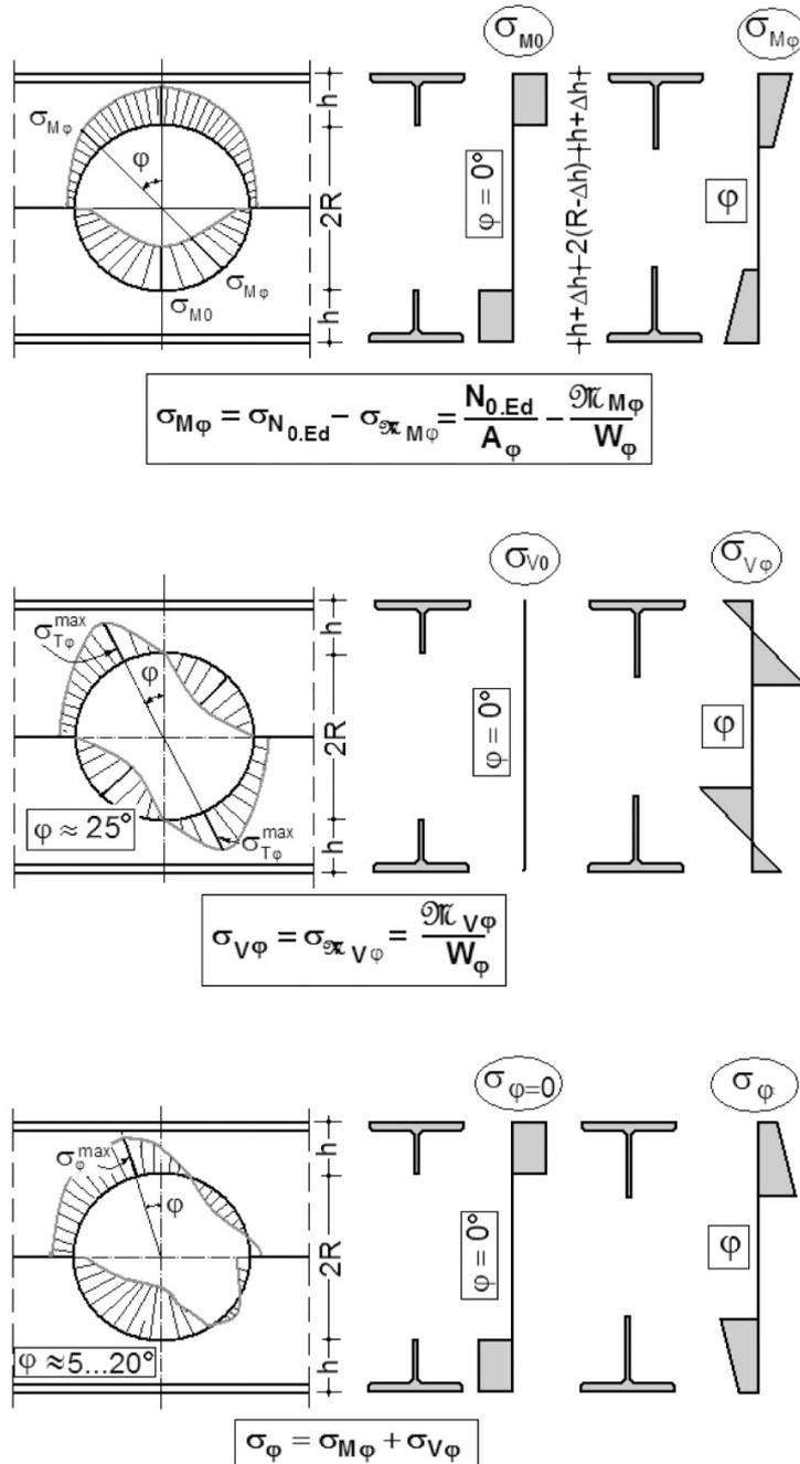
Fig. 10 – State of stresses around the circular hole.
