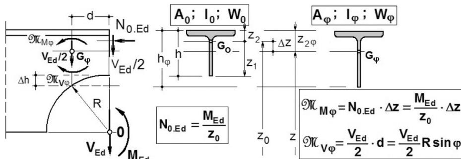
Fig. 9 – Model for the evaluation of the state of stresses.
