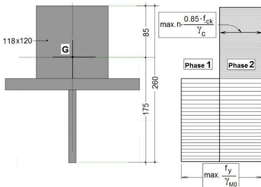
Fig. 8 – Total stresses in the top flange.
