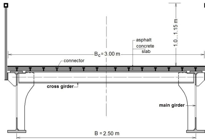
Fig. 1 – Transversal section of the footbridge deck.
