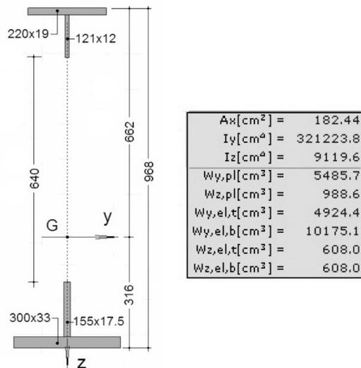
Fig. 3 – Main girder characteristics.
