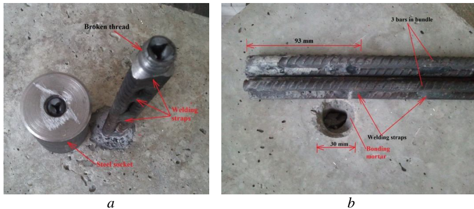
Fig. 6 – Failure modes of some bundled anchors which are embedded 5.5d (93 mm): a – early breaking of the anchor through thread where a threaded couple (socket) is used; b – pulling-out of the anchor from mortar (S-M steel to mortar failure mode) where barrel and wedge gripping system is used; 2 pieces in view.
