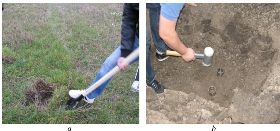
Fig. 3 – The soil sampling in the the natural state: a - scraping the soil, b - introducing in the soil of rings.
