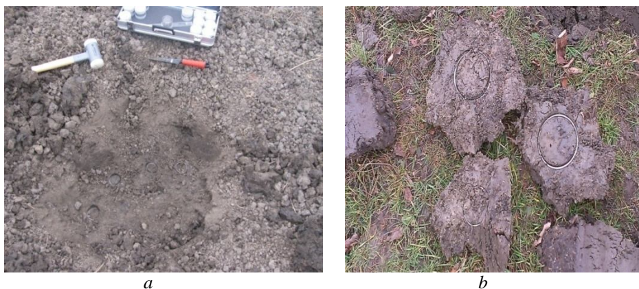
Fig. 4 – Materials necessary sampling: a – hammer, cylinders with caps and spade to extract the cylinders, b – soil with cylinders.
