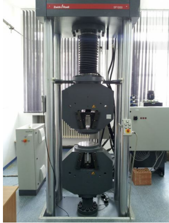
Fig. 7 – Zwick/Roell 100 kN hydraulic test machine.
