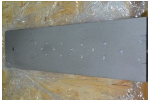
Fig. 1 – Steel plate with bearing balls.
