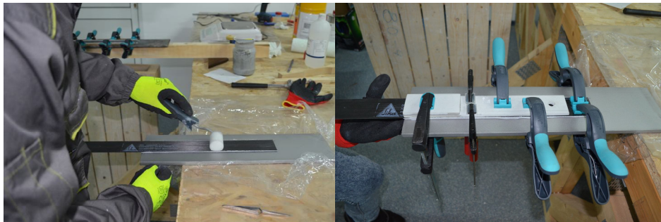
Fig. 3 – Roll-pressing the strip and fixing the specimen.
