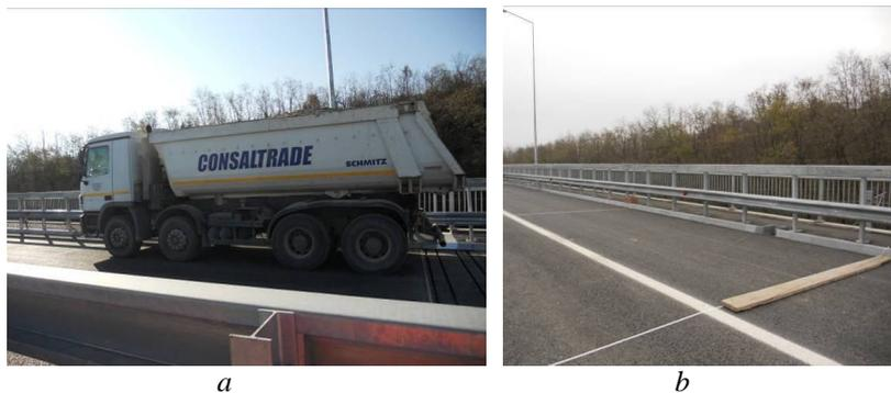
Fig. 4 – *a* – A truck as an excitation source;
