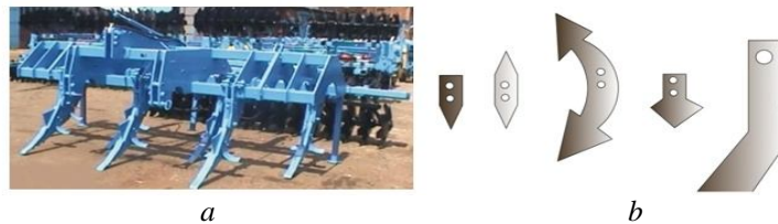
Fig. 5 – Equipment used in the method of loosening soil: a – MAS 7 and b – raising machine with various constructive organs.
