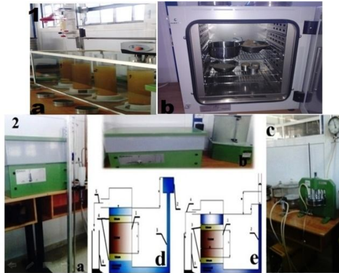
Fig. 2 – The tools used in research: 1: equipment used to analyze the physical properties: a) shaker electromagnetic; b) Eijkelkamp Pipette Apparatus c) drying machine 2: all equipment used in the study of hydraulic properties a) sandbox; b) sand/kaolin box; c) pressure membrane apparatus; d) constant-head method; e) falling head method.
