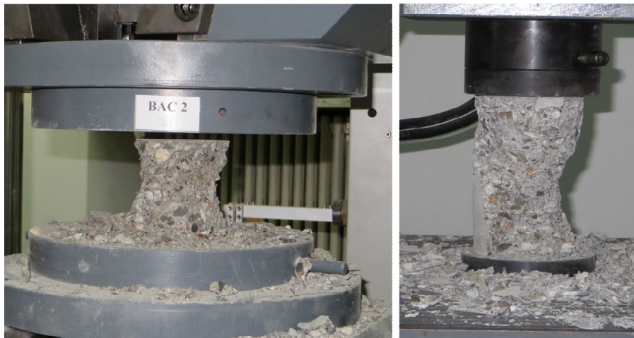
Fig. 4 – Testing cube and cylinder specimens.
