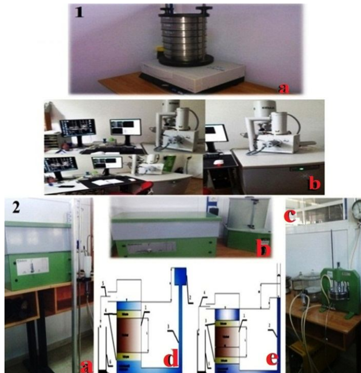
Fig. 2 – The tools used in research: 1: equipment used to analyze the morphology of mineral particles: a – shaker electromagnetic; b – equipment used in microscopic analysis SEM 2: all equipment used in the study of hydraulic properties: a – sandbox; b – sand/kaolin box; c – pressure membrane apparatus; d ) constant-head method; e ) falling head method.
