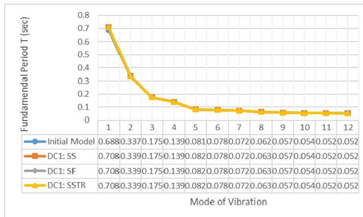
Fig. 5 – Damage Case 1: Modal response of the updated models.
