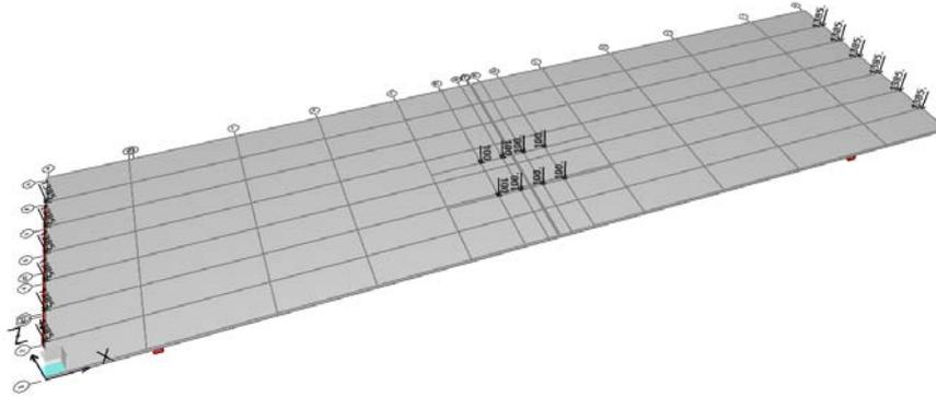
Fig. 2 – Finite Element model of bridge structure, and applied loads.
