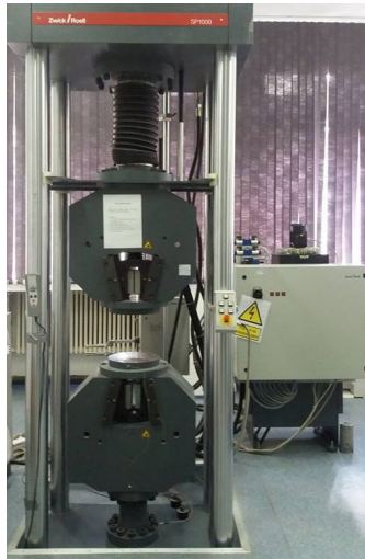
Fig. 11 – ZWICK/ROELL 100 kN hydraulic test machine.
