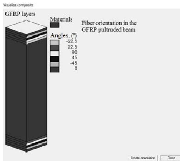
Fig. 5 – Defining of the composite material for the numerical modelling.
