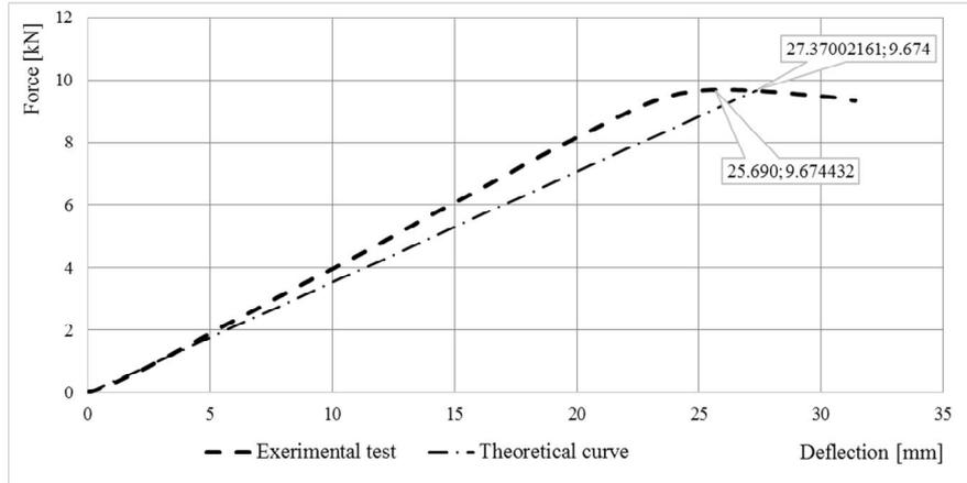
Fig. 2 – Force-deflection curve of the pultruded I beam made of GFRP  $120 \times 60 \times 6$ .
