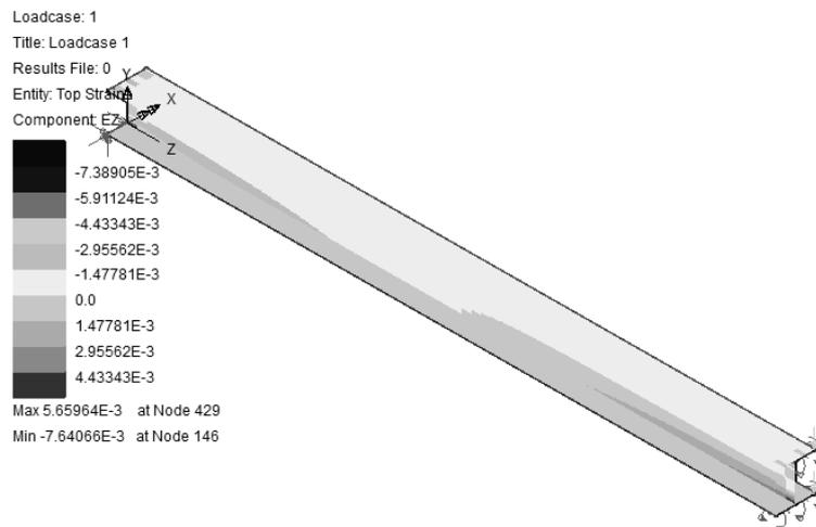
Fig. 8 – The tensile strain at the tensioned bottom of the GFRP flange.
