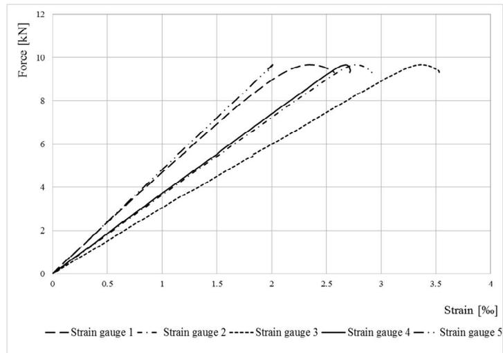
Fig. 3 – Tensile strain levels at the bottom flange of the GFRP ‘T’ profile.
