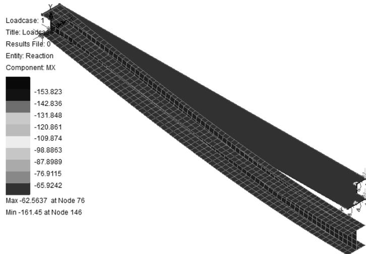
Fig. 7 – The flexural strength at the bottom of the GFRP flange.
