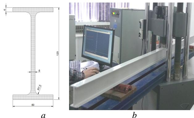
Fig. 1 – GFRP pultruded beam: *a* – cross section dimensions; *b* – test program.
