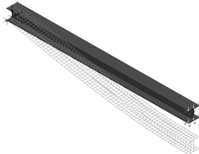
Fig. 6 – Deformed mesh of the GFRP beam.
