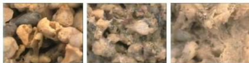
Fig. 4 – Assessment of the intervention measures, investigated with the FOM technique (on the left – untreated area; in the middle and on the right – areas treated with solutions intended to reduce porosity) (Moropoulou et al. , 2013).
