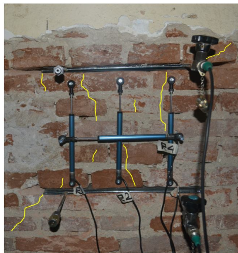
Fig. 6 – Crack development in masonry during two flat jacks test.
