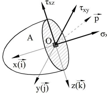
Fig. 3 – Stress components in a  $x$ - $y$ - $z$  Cartesian coordinate system (Mazilu, 1977).
