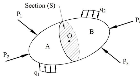
Fig. 1 – Body in equilibrium under an arbitrary system of forces (Mazilu, 1977).
