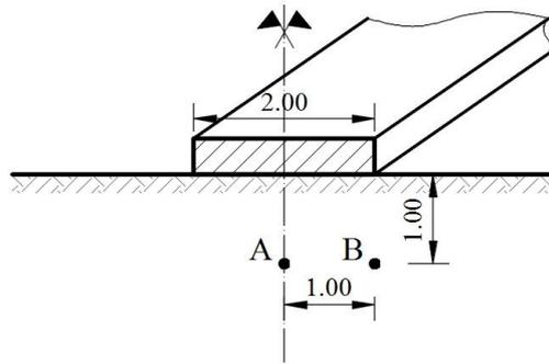
Fig. 11 – Position of the two points in which the stress state is calculated.
