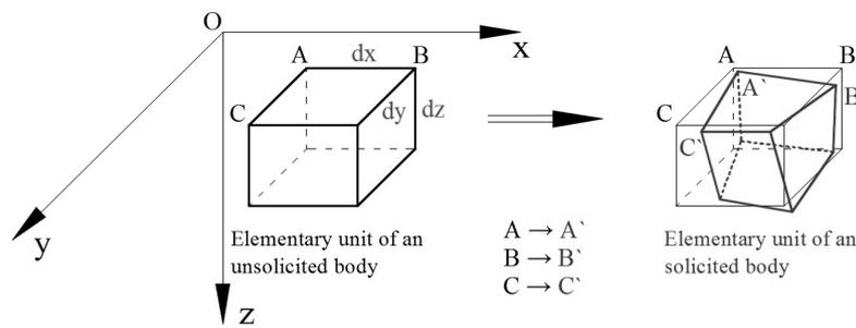
Fig. 7 – Displacement and deformation of an elementary unit of a body (Das, 2008; Budhu, 2000).
