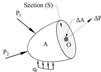
Fig. 2 – Stress development in point  $O$  of surface  $S$  (Mazilu, 1977).
