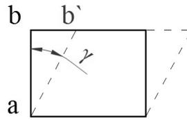
Fig. 10 – Definition of shear strain (Budhu, 2000).
