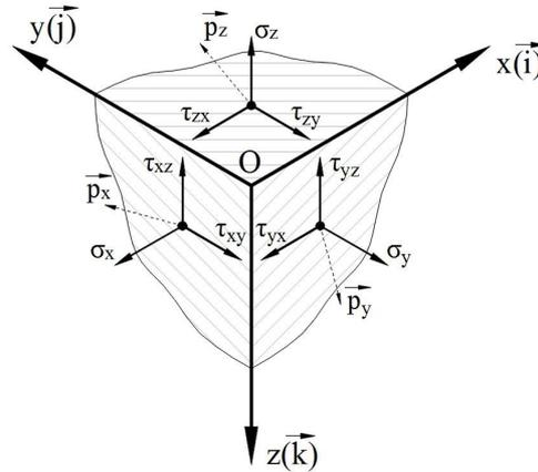
Fig. 4 – Stress components in three dimensions (Mazilu, 1977).
