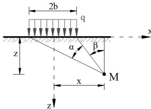
Fig. 13 – Parameters involved in the stress state calculation (Aysen, 2005; Craig, 2004; Das, 2008).
