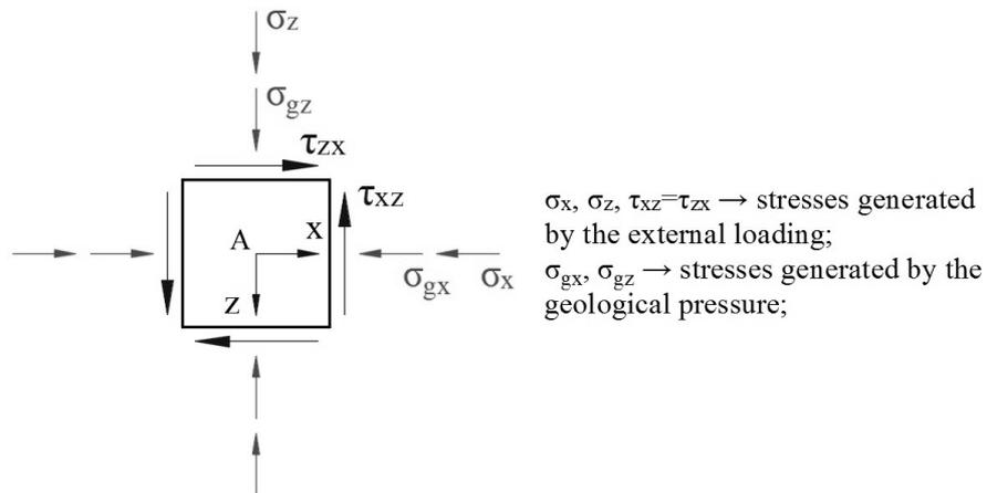
Fig. 12 – Plane state of stress in a point in the soil mass.
