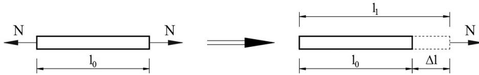
Fig. 9 – Definition of normal strain, (Hosford, 2010).
