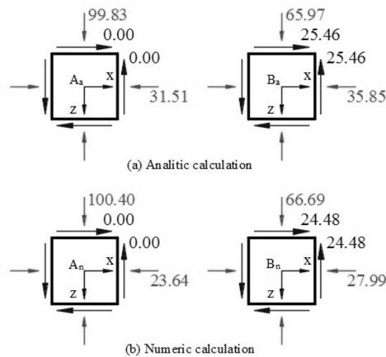
Fig. 15 – Results from analytical and numerical calculation for points A and B, [kPa].
