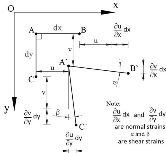
Fig. 8 – Strain components in the  $xy$  plane (Das, 2008; Hosford, 2010).
