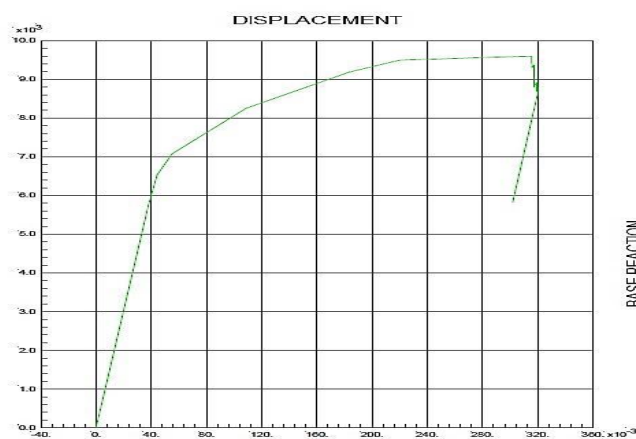
Fig.7 – Lateral force- top displacement curve, the case of progressive horizontal loads on the Y direction.
