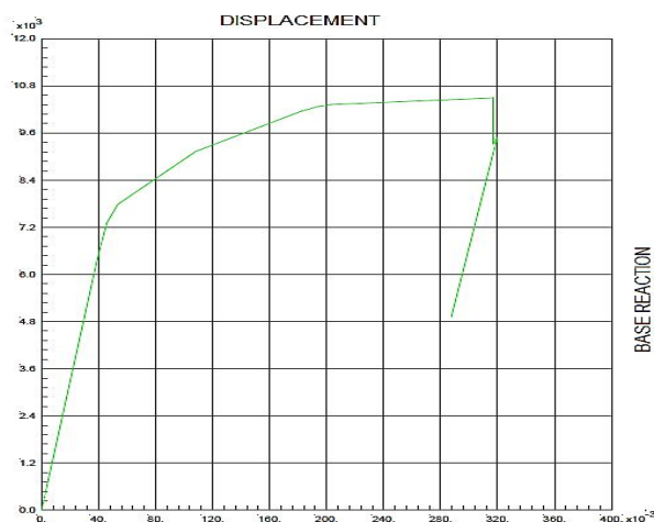
Fig. 6 – Lateral force- top displacement curve, the case of progressive horizontal loads on the X direction.
