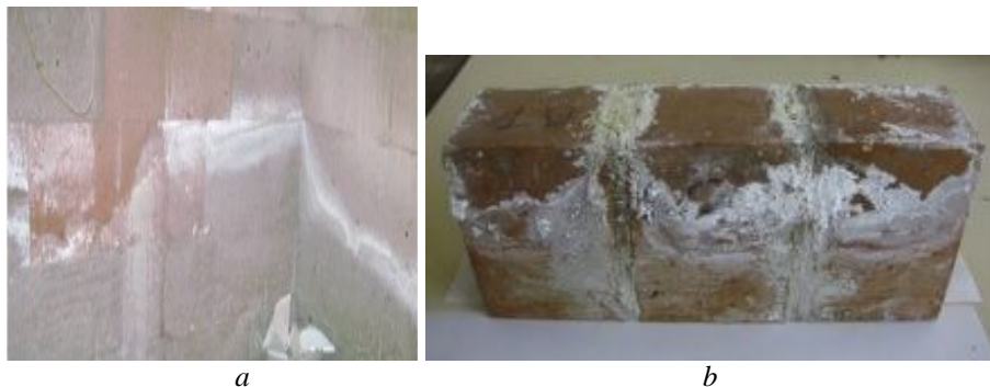
Fig. 12 – a – Efflorescences (Korkane, 2013); b – Crystallized salts (Gentilini et al. , 2012).
