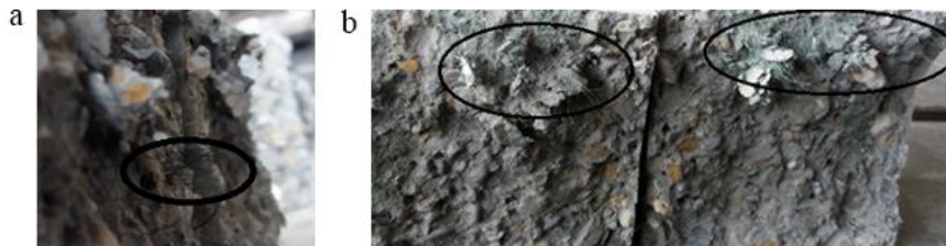
Fig. 4 – Fiber distribution in concrete.
