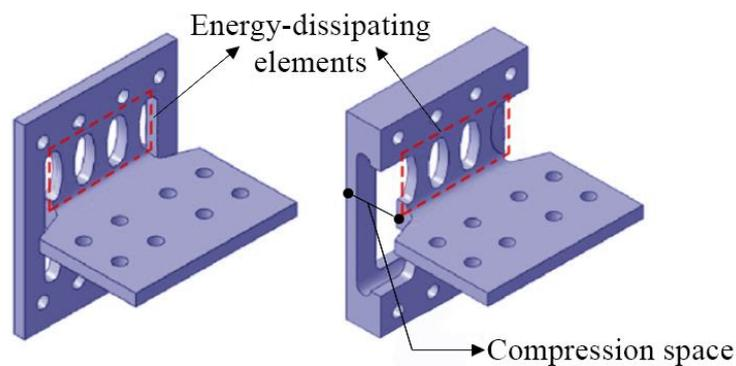
Fig. 7 – Cast DST elements (Tong, L. *et al.*, 2016).
