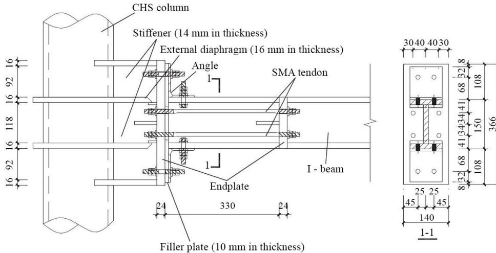
Fig. 12 – SMA tendon connection for circular columns (Wang *et al.*, 2015).
