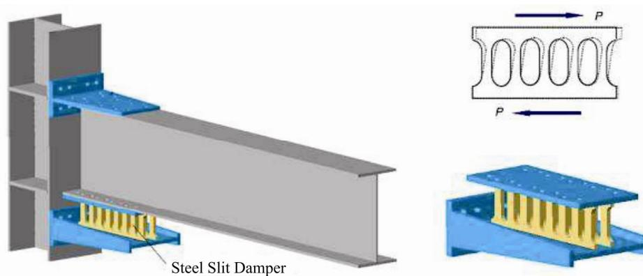
Fig. 3 – Steel slit damper connection (Oh *et al.*, 2009).
