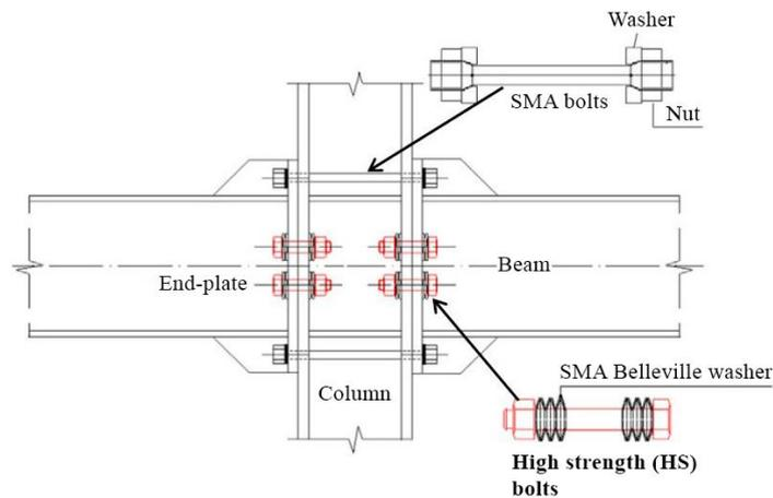
Fig. 11 – SMA tendon connection (Yam *et al.*, 2015).
