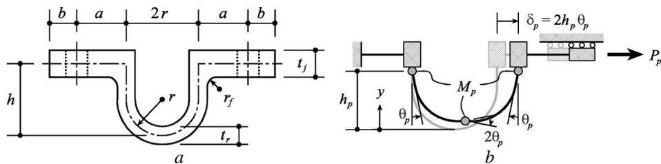
Fig. 2 – PI dissipative element: a. geometric characteristics, b. failure mechanism (Koetaka *et al.*, 2005).
