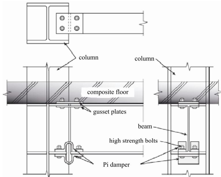
Fig. 1 – Connection with PI damper (Koetaka *et al.*, 2005).
