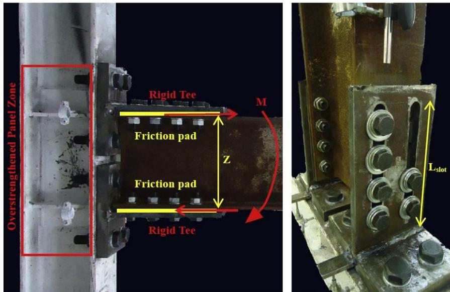
Fig. 14 – Friction damper connection (Latour *et al.*, 2015).
