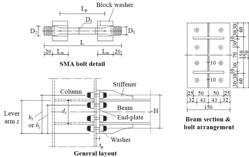
Fig. 10 – SMA bolt connection (Yam *et al.*, 2015).
