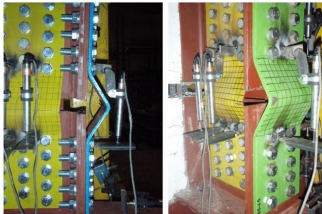
Fig. 9 – Damaged dissipative bolted fuse connection (Calado *et al.*, 2013).
