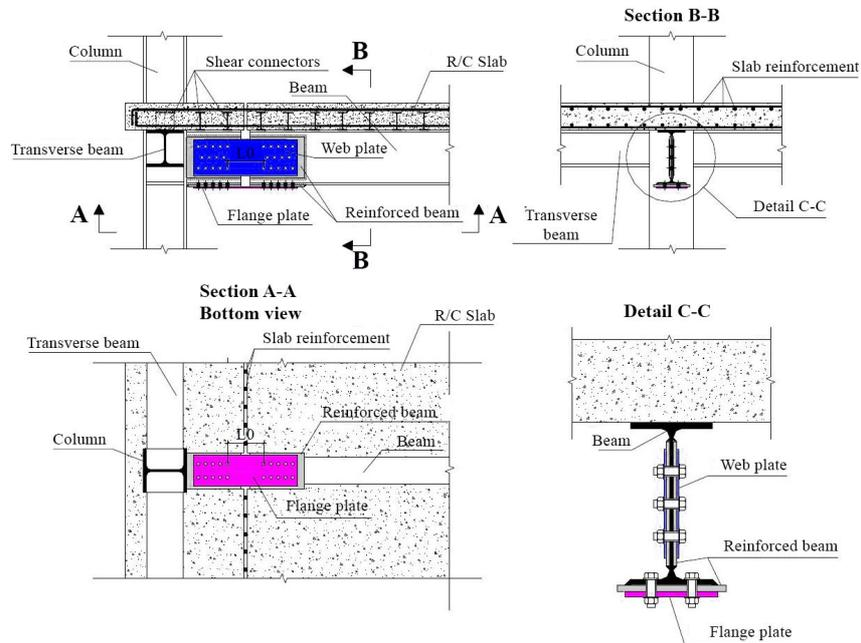
Fig. 8 – Dissipative bolted fuse connection (Calado *et al.*, 2013).
