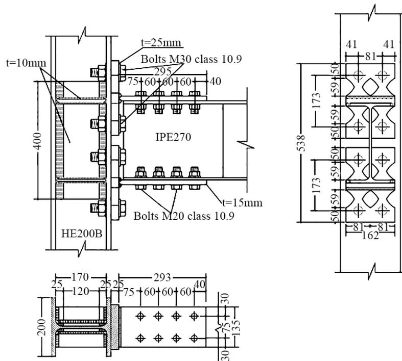
Fig. 6 – DST connection with hourglass shaped end plate (Latour & Rizzano, 2015).
