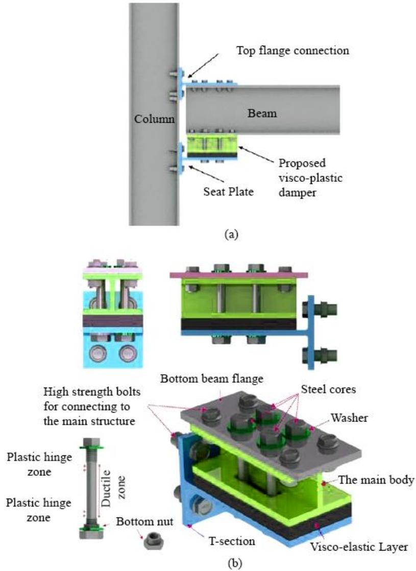
Fig. 13 – Visco-elastic and hysteretic dampers connection: *a* – overall view; *b* – detail (Banisheikholeslami *et al.*, 2016).
