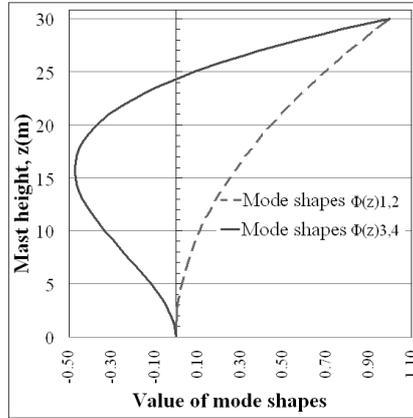
Fig. 2 – First and second mode shapes of the 30 m high steel mast.
