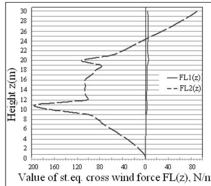
Fig. 5 – Cross wind forces for first and second modes of the 30m high steel mast, generated by vortex shedding.
