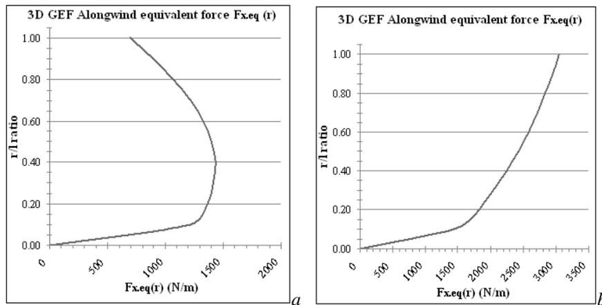
Fig. 4 – Equivalent static force for displacement effect ( $e = d$ ): *a* – for real 30 m lighting mast with variable mass and cross-section and *b* – for a 30 m mast with constant mass and cross-section  $v = 33.5$  m/s.
