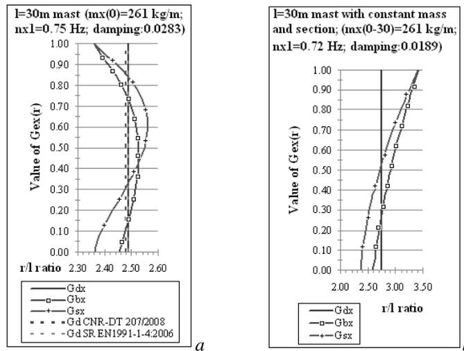
Fig. 3 – Gust Effect Factor for displacement ( $e = d$ ), bending moment ( $e = b$ ), shear force ( $e = s$ ) in the alongwind direction: *a* – for the real 30m mast; comparison with EU, Italian codes and *b* – for a 30m mast with constant mass and cross-section.
