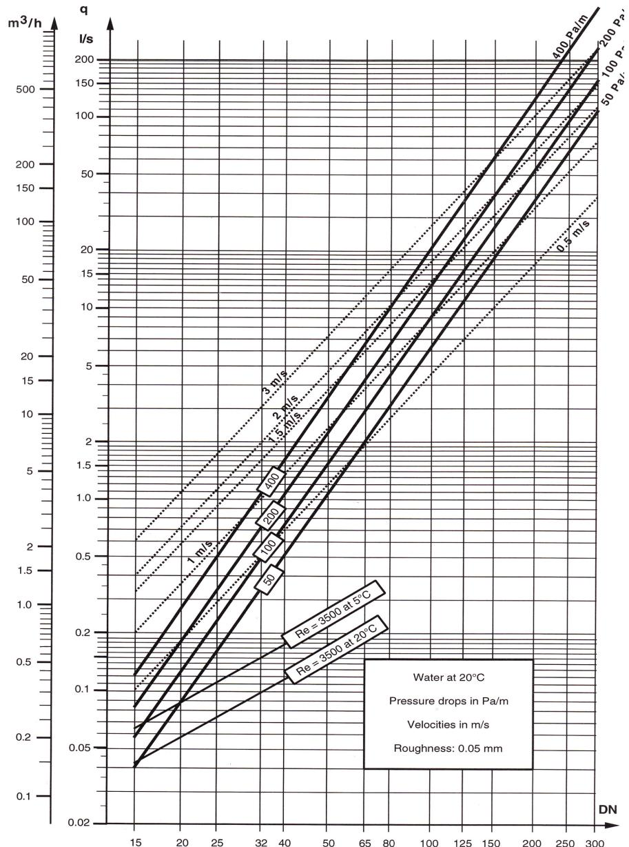
Fig. 1 – Pressure drops and velocities in pipes.
