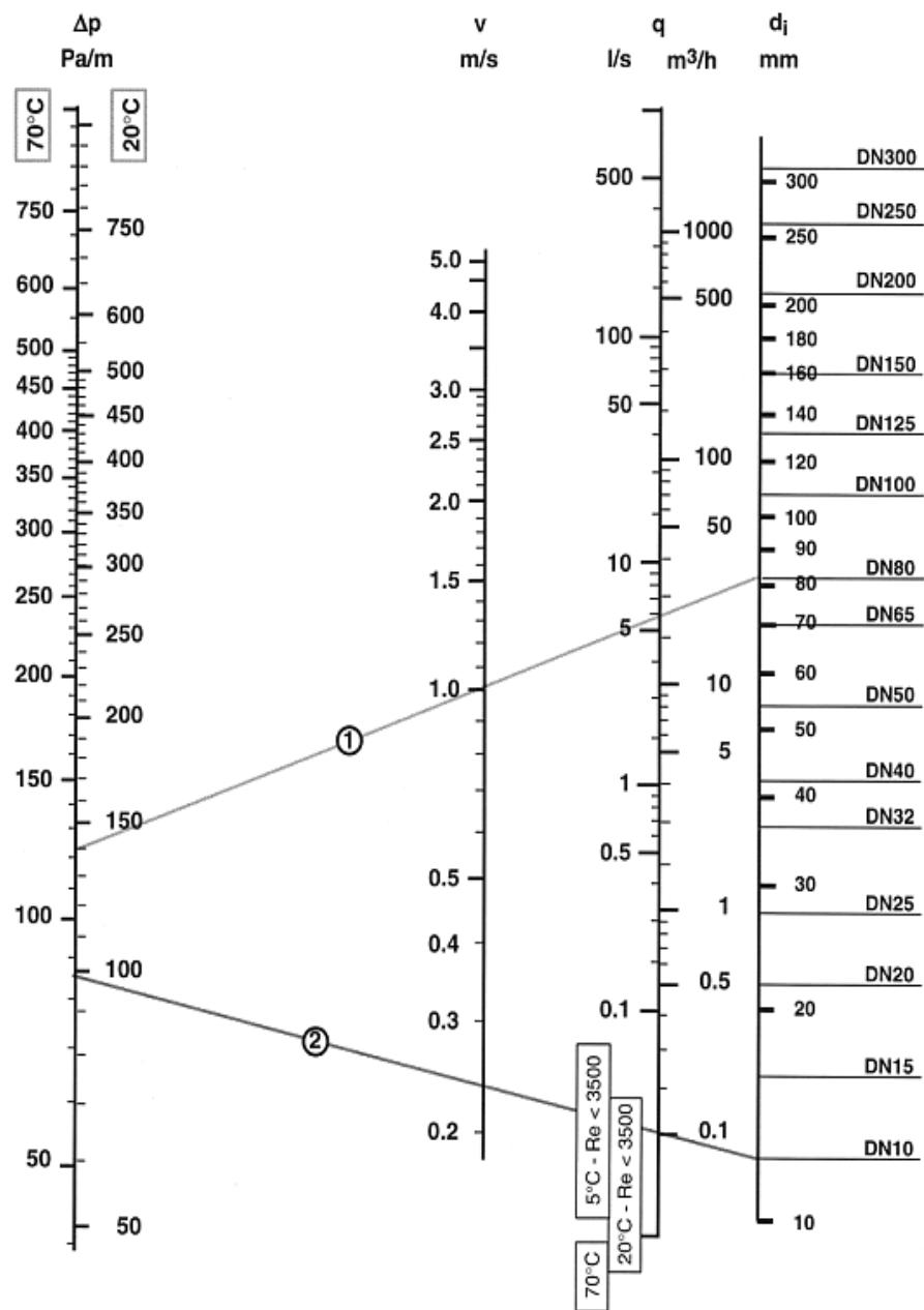
Fig. 2 – Pressure drops and velocities (pipes with a roughness of 0.05 mm) for water at  $20^\circ\text{C}$  and  $70^\circ\text{C}$ .
