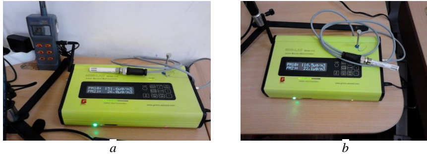
Fig. 4 – Mini Laser Aerosol Spectrometer (Mini-LAS) installed in a) classroom I-16 (no ventilation) b) classroom I-17 (with ventilation).
