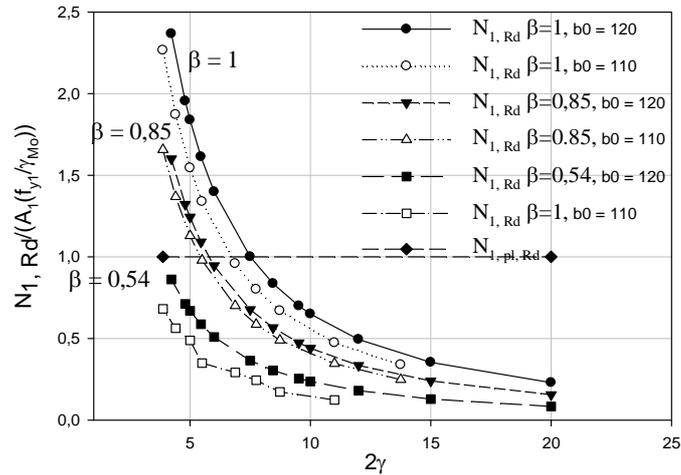
Fig. 3 – Chord plasticization failure for different  $\beta$ .
