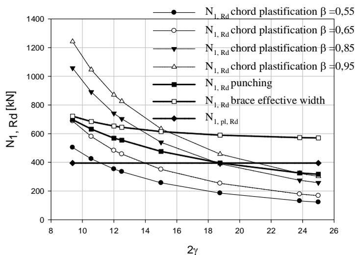
Fig. 5 – Comparison between chord plasticisation, punching shear and effective width resistance.
