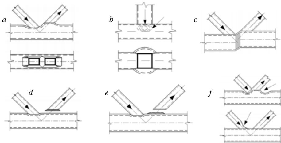
Fig. 2 – Failure modes in K-Connections according to EN 1993-1-8: *a* – chord face failure; *b* – chord side wall failure; *c* – Chord shear failure; *d* – Punching shear; *e* – brace failure; *f* – local buckling.
