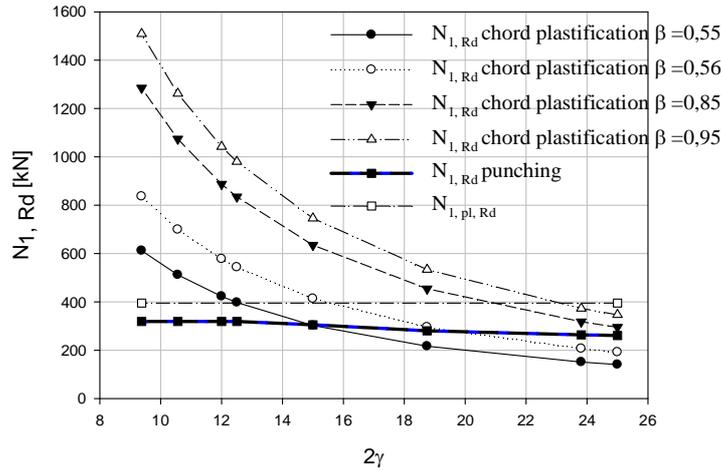
Fig. 6 –  $N_{1, Rd}$  chord plastification, punching shear and effective with resistance for slender braces.
