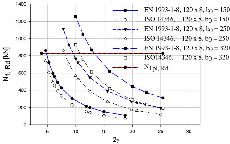
Fig. 7 –  $N_{1, Rd}$  chord plastification, comparison EN 1993-1-8 (2006) with ISO 14346 (2013)
