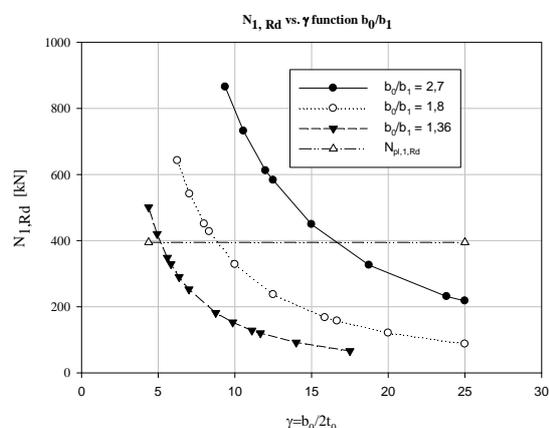
Fig. 4 – Effective width failure function of bracing to chord ratio.
