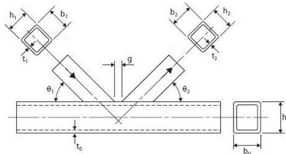
Fig. 1 – Gap joint: notations.
