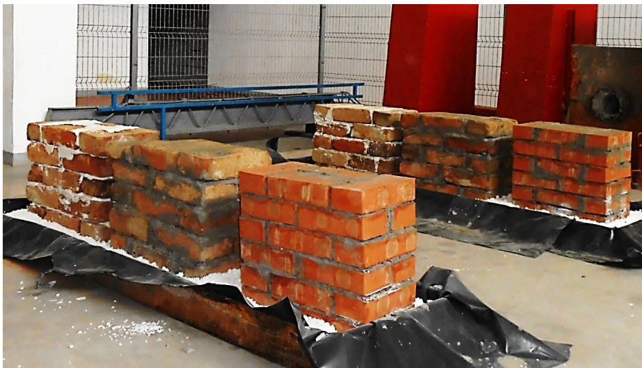
Fig. 1 – Brick masonry walls.
