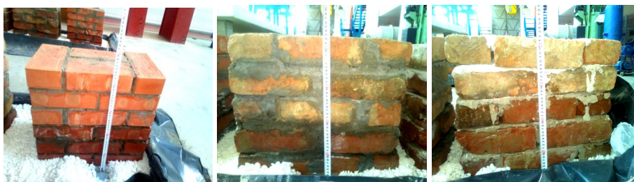
Fig. 2 – Measuring the ascensional moisture level
