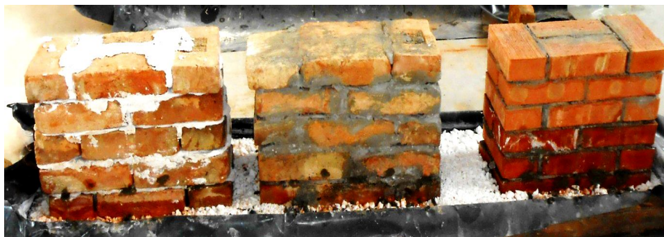
Fig. 3 – Masonry walls treated for water-proofing.
