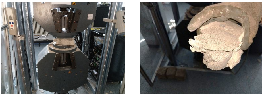
Fig. 3 – The failure modes of concrete bricks with VCH filled with cement mortar at 14 days.
