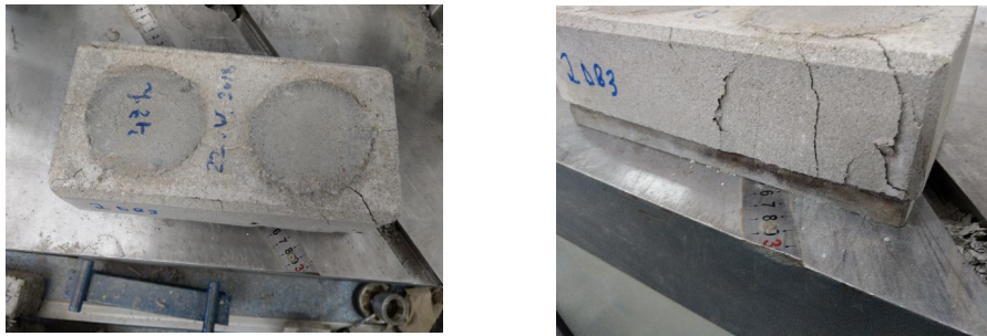
Fig. 2 –The failure modes of concrete bricks with VCH filled with cement mortar at two days.
