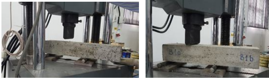
Fig. 3 – The placing of the A, respective B prisms on the machine steel plates for the bending test.
