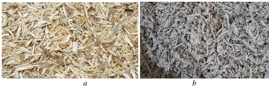
Fig. 1 – Wood chips used for the prisms obtaining: a – the dry wood chips; b – the mixture of concrete with wood chips.
