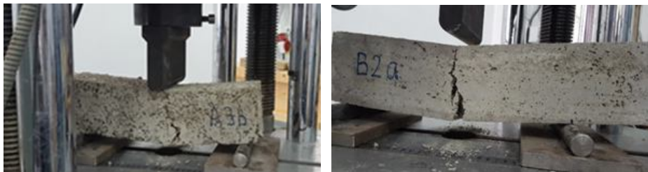
Fig. 4 – The failure of the A and B specimens under three-point bending test.
