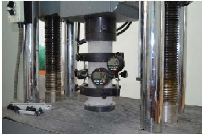
Fig. 1 –Experimental test in compression of concrete with chopped PET.
