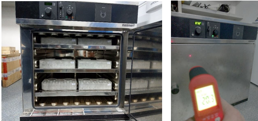
Fig. 2 – Placing of the specimens in the oven (left) and keep them at + 70°C for 48 hours (right).
