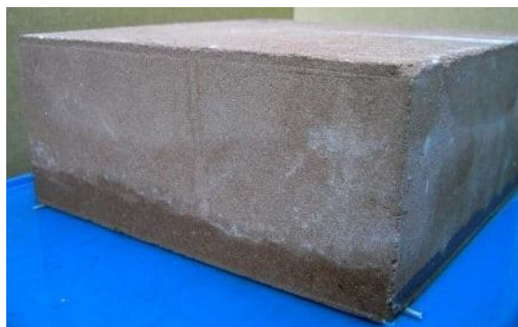
Fig. 7 – Capillary absorption in concrete block.
