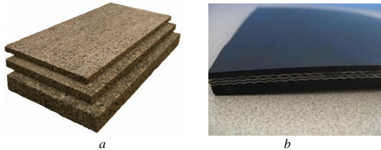
Fig. 15 – Materials used for vibration dissipation: a – cork insulation; b – rubber band .
