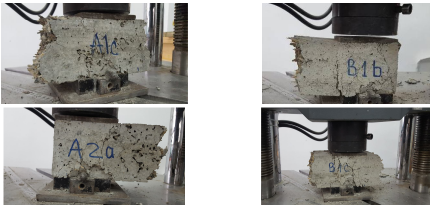
Fig. 2 – The failure of the A (left) and B (right) specimens under compressive
