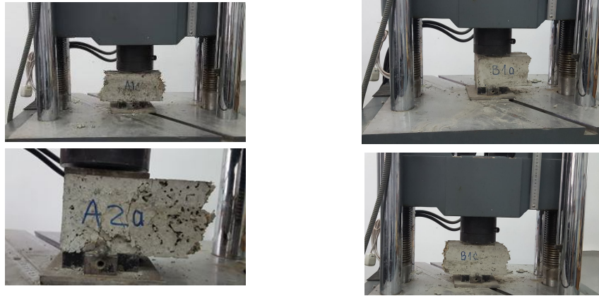
Fig. 1 – The placing of the A (left), respective B (right) prisms on the machine steel plates for the compressive test.
