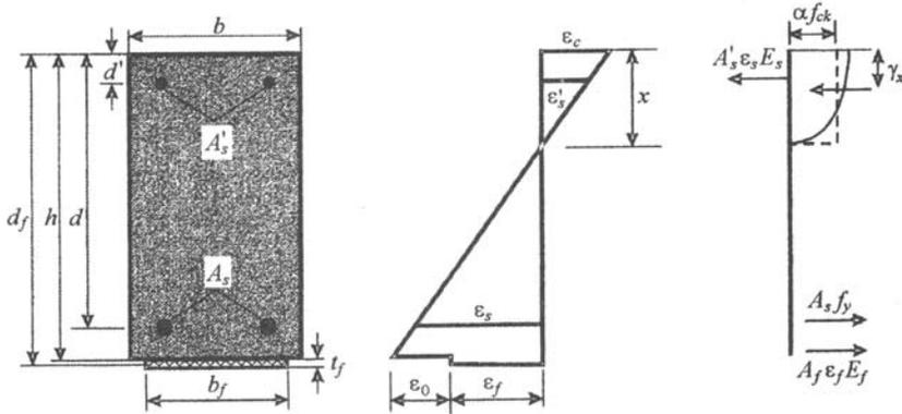
Fig. 6.– Strain and stress distribution on a composite section subjected to bending at the ultimate limit state.
