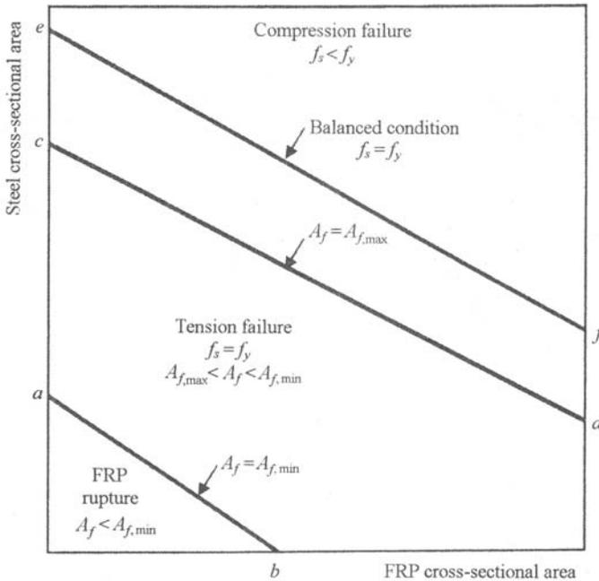
Fig. 5.- Schematic illustration of failure modes for the strengthened beam [2].
