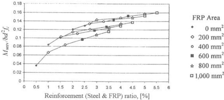
Fig. 11.- Reinforcement ratio vs. service moment curves.
