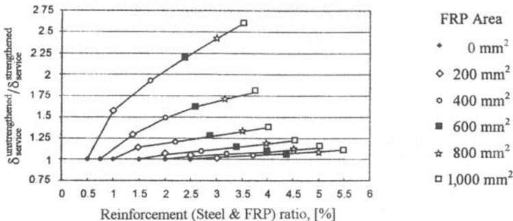
Fig. 9.- Reinforcement ratio vs. deflection curves.
