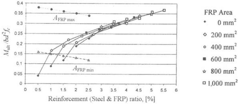
Fig. 10.- Reinforcement ratio vs. ultimate moment curves.
