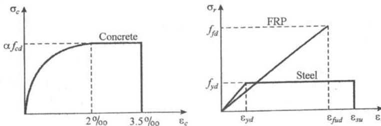
Fig. 4.– Material models at ultimate limit states.
