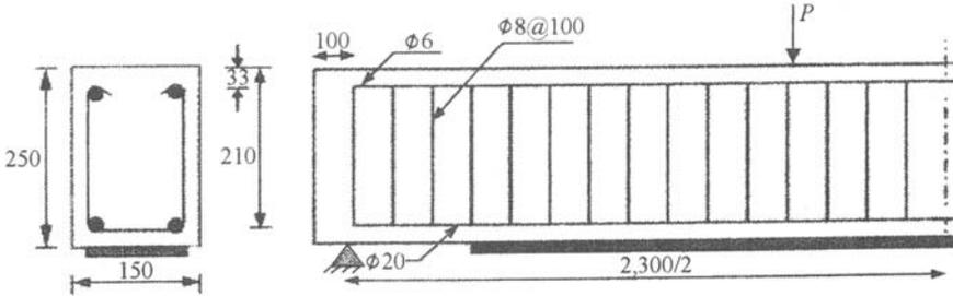
Fig. 7.- Beam geometry and reinforcement.
