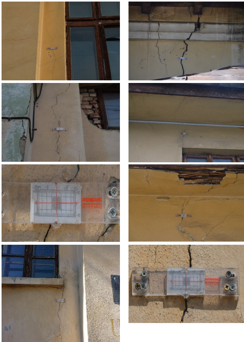
Fig. 9 – Rulers placement to cracks evolution's monitoring.
