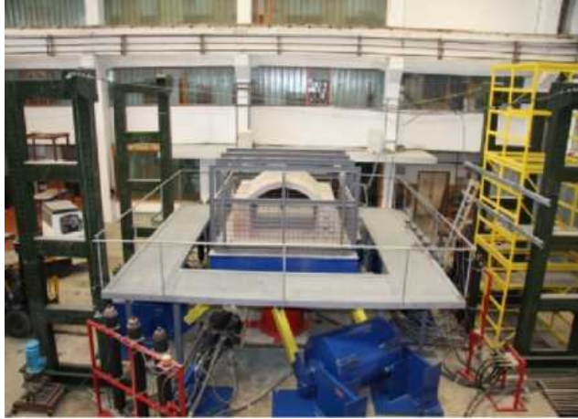
Fig. 4 – ANCO R250-3123 tri-axial vibration shake table.
