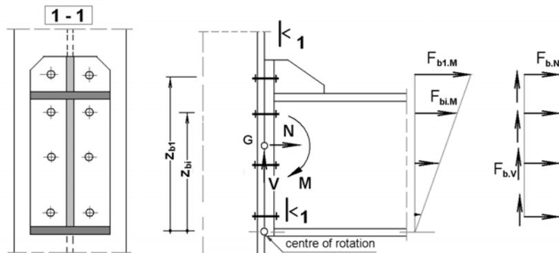
Fig. 1 – Connection with end plate and bolts.
