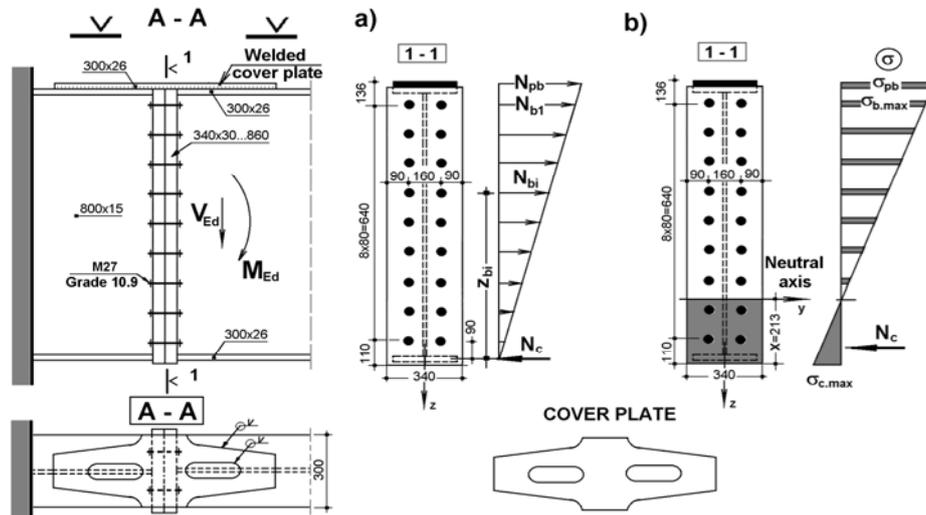
Fig.10 – Connection with end plates and a cover plate.
