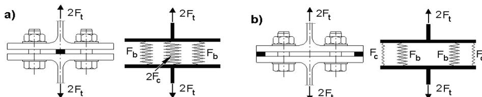
Fig. 3 – Parts of contact area.
