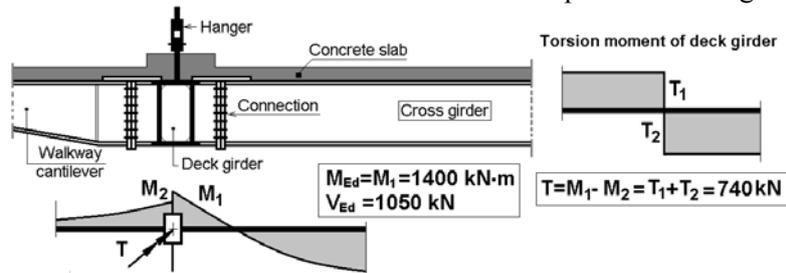
Fig. 8 – The constructive scheme of the connection and calculated forces.
