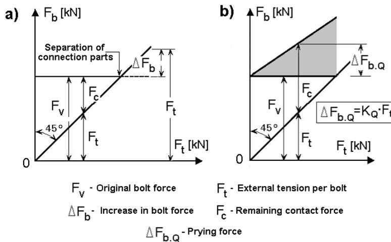
Fig. 4 – Effect of the location of the contact pressure on the bolt force.
