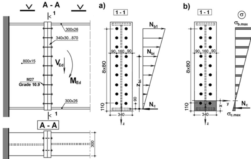
Fig. 9 – Connection with end plates and no additional cover plates.
