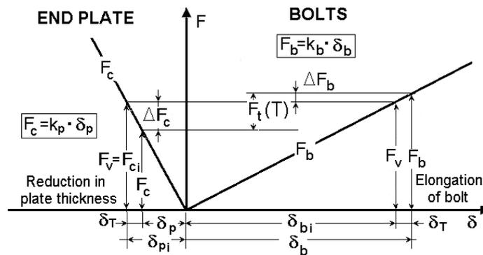
Fig. 2 – Forces in prestressed fastener before end plates separate.
