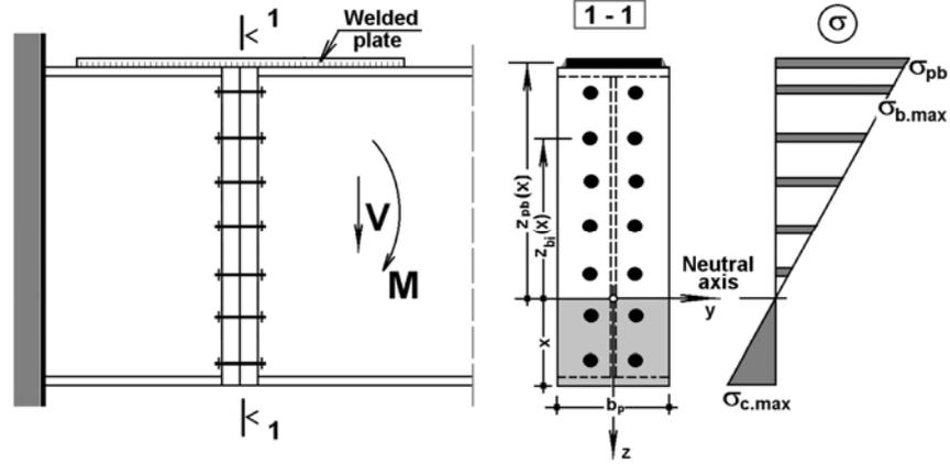
Fig. 6 – Connection made with an end plate and a cover plate welded to the tension flange.
