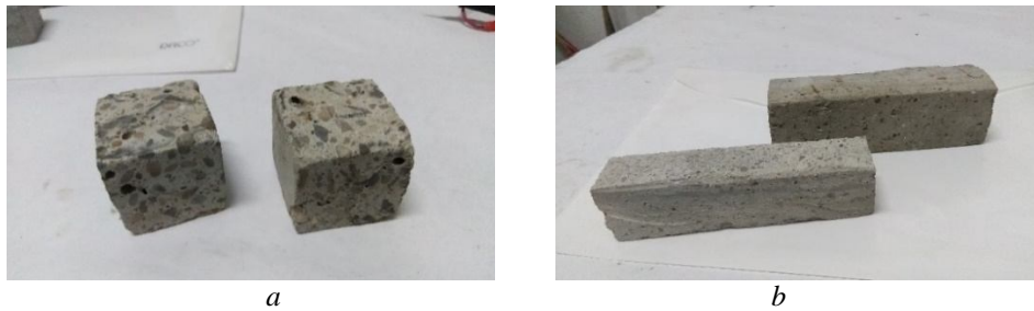
Fig. 13 – Test specimens: a – concrete samples; b – shotcrete samples.
