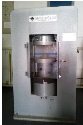
Fig. 15 – Compressive strength test – concrete.
