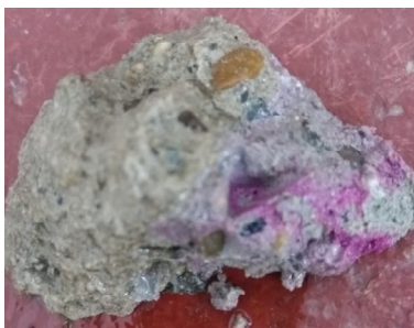
Fig. 10 – Concrete's carbonation test.
