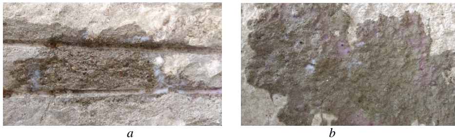
Fig. 8 – Alkalinity test performed in-situ.
