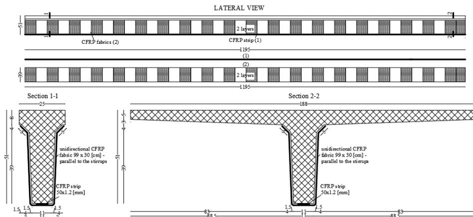
Fig. 8 – CFRP consolidation – discrete strips
