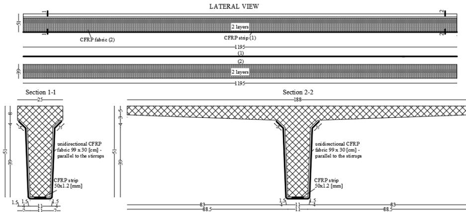
Fig. 6 – CFRP consolidation – continuous jacketing
