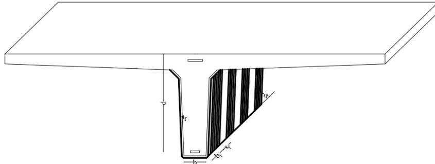
Fig. 7 – CFRP sheet – discrete strips.
