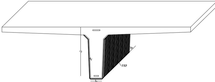
Fig. 5 – CFRP sheet - continuous jacketing
